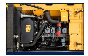
The water cooled, 4 cycle diesel, 6 cylinder in line, direct injection turbocharged engine is built for power, reliability,
