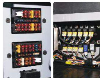
Compact fuse box for easy inspection
