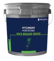
Dark grey, multipurpose EP grease primarily designed where an extra measure of protection in shock loading condition is required. Contains a highly refined mineral base oil, EP additives, rust and oxidation inhibitors, plus molybdenum disulphide solid film lubricant.
