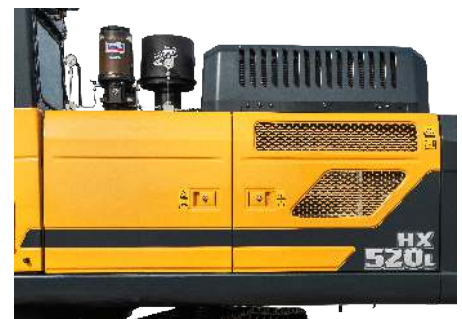
ENLARGED AIR INLET WITH GRILL COVER
