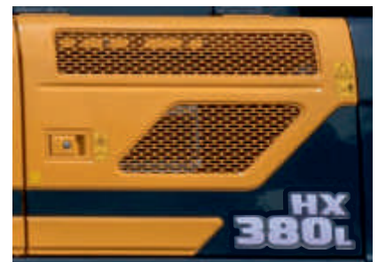
Enlarged Air Inlet with Grill Cover
