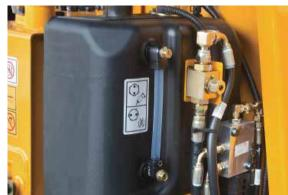
Selector Valve for Single or Double Acting Piping
