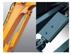
Cylinder Covers Standard boom and dozer cylinder covers provide added protection.
