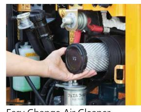
Easy Change Air Cleaner The R30Z-9AK is equipped with a durable plastic air cleaner designed for easy maintenance.
