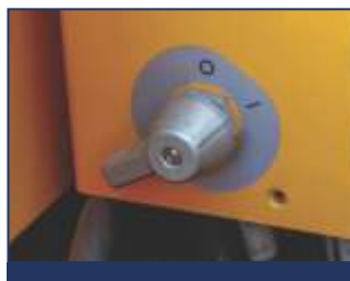
BATTERY DISCONNECT SWITCH
