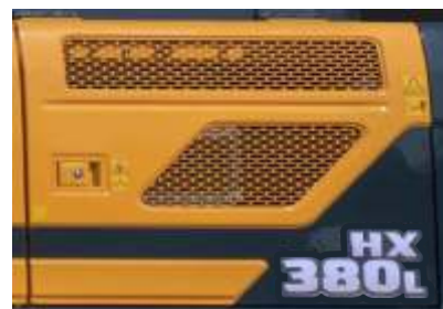
Enlarged Air Inlet with Grill Cover
