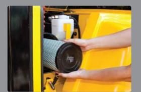
**Easy Change Air Cleaner**The air filter is readily accessible for cleaning or replacement.
