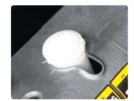
Brake Fluid Reservoir with Level Switch
